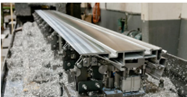
Milling of sliding table surface
