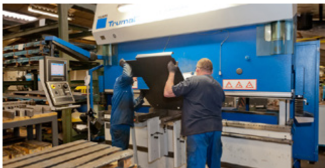
Computer assisted steel plate bending
